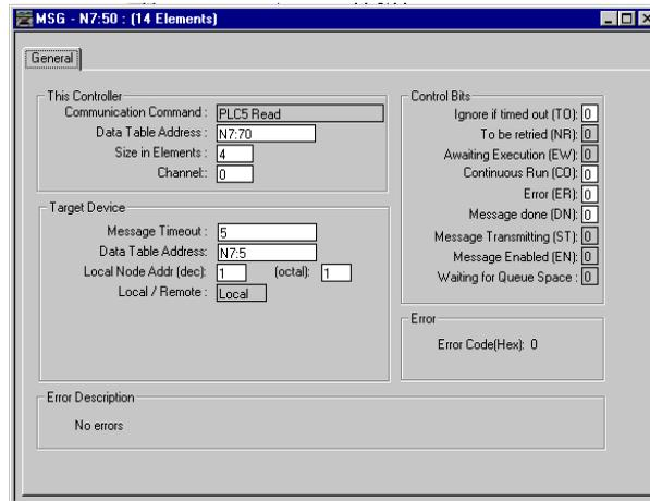
**2** In the General tab of the MSG dialog box, refer to the This Controller group. In the Data Table Address field, select the area of PLC memory to use in the read/write transaction with the inverter.
