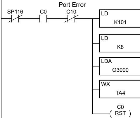
This rung writes values to the SC-OPE. We are loading the values from V3000 in the DL250 CPU and moving them into TA4 (V4). The equivalent MODBUS address = 40005.
