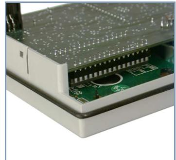
**4** Insert the SC-OPE into the bezel/housing. You can use the square modular connector and corresponding opening to verify the orientation of the two parts. Begin with the SC-OPE bottom edge as shown (below, left), engaging the two internal latches at the bottom of the bezel/housing.
