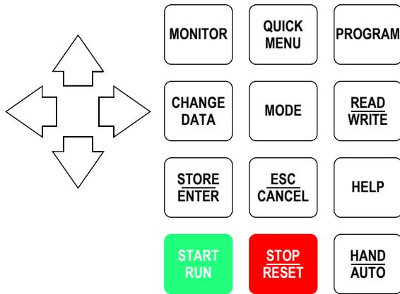
For example, press the Program key to display its name on the third display line.
