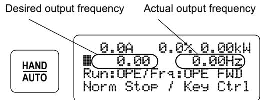
3 Press the Change Data key to edit the desired inverter frequency setting. The “>” and “<” characters indicate Change Data is active.
