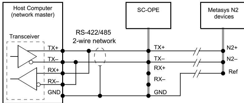
Remember to add a termination resistor at each physical end of the network, or verify that the device at the end has internal termination. Bias resistors are also important. See “Network Termination” on page 4-8.
