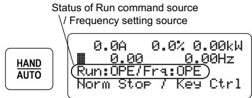
In Monitor mode, the second line displays the desired and actual frequencies. You can edit the desired frequency in Monitor Mode, setting parameter F001 (Frequency Setting) in the inverter.
