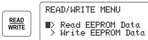
**3** With the read operation selected, press Store/Enter to perform the Read EEPROM Data. After a few seconds the SC-OPE displays the confirmation message as shown.
