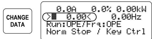
4 Use Right and Left Arrow keys to move the cursor to the digit you want to change. Then use the Up and Down Arrow keys to increment or decrement the digit. This example uses 10Hz. We recommend using a relatively slow initial speed.
