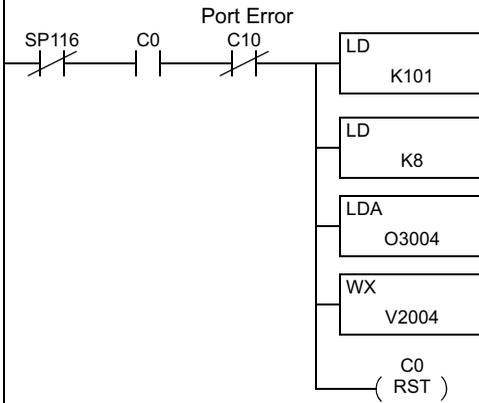
This rung writes values to the SC-OPE. We are loading the values from V3004 in the DL250 CPU and moving them into V2004 in the inverter.
