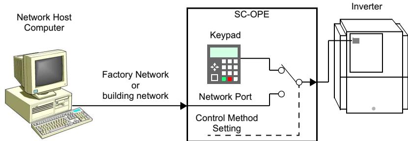
**Hand/Auto Setting** When receiving and interpreting network write commands, the SC-OPE will command the inverter as if an operator were using the SC-OPE (from the inverter’s point of view). If the inverter is configured for control via its own keypad or input terminal, it will ignore network commands sent via the SC-OPE. So, controlling the inverter from a network requires that you set the following:
