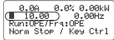
6 Press the Start Run key. The RUN LED should turn ON to indicate the inverter is in Run Mode. The monitor screen will indicate the actual frequency, motor direction and status such as “Ramp Up,” “Const Spd,” “Ramp Down,” and “Norm Stop.”
