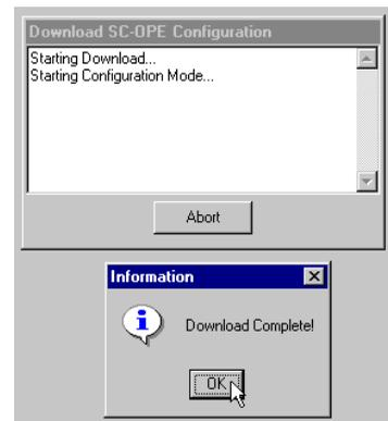
When you have changed the inverter type in a configuration (such as from “L100” to “SJ100”), a configuration download includes inverter-specific firmware for the SC-OPE. The status message “Starting Flash Download Mode” followed by “Buffer 1 of 8” etc. indicates the new inverter-specific firmware is downloading. The SC-OPE shows the buffer (block) number which is currently loading.
