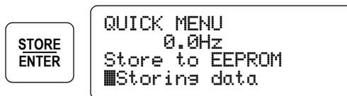
When completed, the parameter values will then be in the EEPROM, used in the next powerup of the inverter.
