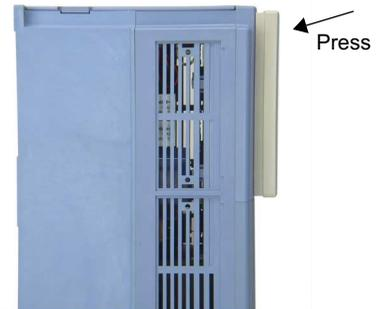
**7** To remove the SC-OPE from the inverter, press the retention latch at the top on the SC-OPE housing. One technique is to grasp the SC-OPE at the bottom edge and use the thumb to press the retention latch as shown.
