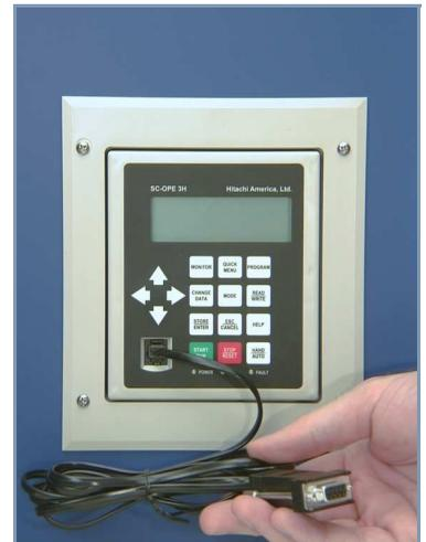
**Note:** The SC-OPE will communicate with its Configuration Editor in a PC via the RS-232 port. Do not attempt to use the Configuration Editor over a factory network.
