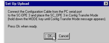
At this point the Editor will attempt to communicate with the SC-OPE and upload its current configuration to the PC. If the upload is successful, you'll see the confirming messages below.
