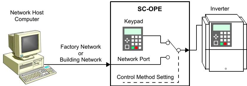
The SC-OPE's control method setting is fundamental and very important to know. Its default setting is "Keypad Control," displayed in Monitor Mode in the corner
