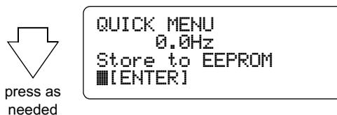
4 Press the Store/Enter key to move (store) parameters from the inverter's RAM to its EEPROM. The status "Storing data" displays for a few seconds.
