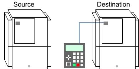
**Note:** Do not run the motor; the inverter cannot update all of its parameters while it is in Run Mode.
