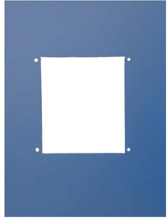
**2** Place the gasket (included in the Bezel Kit) around the inside perimeter of the bezel/housing as shown. Align the holes in the gasket with the ones in the corners of the bezel/housing. This gasket provides a seal between the bezel/housing and the panel's front surface.
