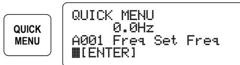
3 Press the Down Arrow key as needed to reach the bottom of the Quick Menu list for the Store to EEPROM menu item (or press the Up Arrow key once; the list navigation is also rotary in design).
