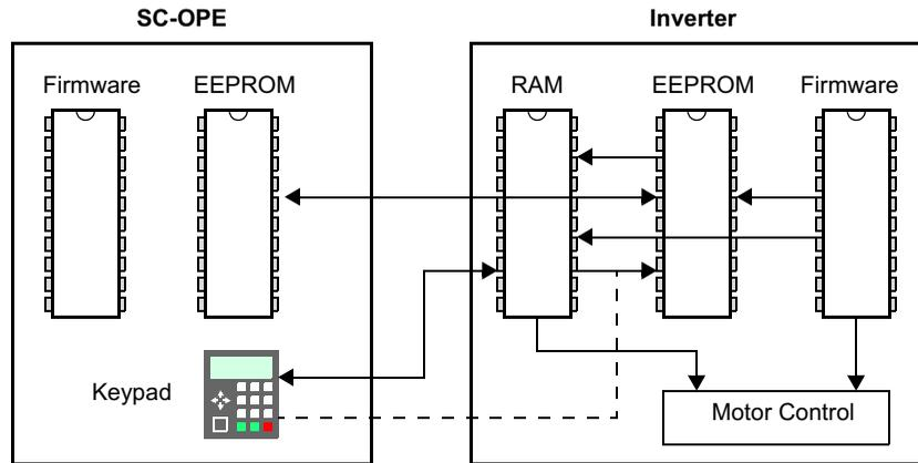
The SC-OPE and inverter memory resources operate according to the following:
