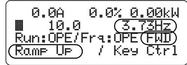
7 Press the Stop/Reset key. The example motor profile below shows the keypad command of motor operation. The Up Arrow and Down Arrow keys adjust the motor speed (when the inverter frequency source is configured as the operator keypad — SC-OPE).
