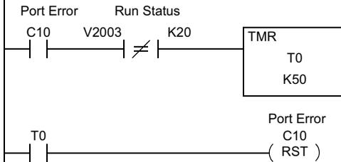
Keep reading the run status register until the comm error clears between the SC-OPE and the Drive. K20 is the value of the run status register when there is an error for SC-OPE-to-inverter communications.
