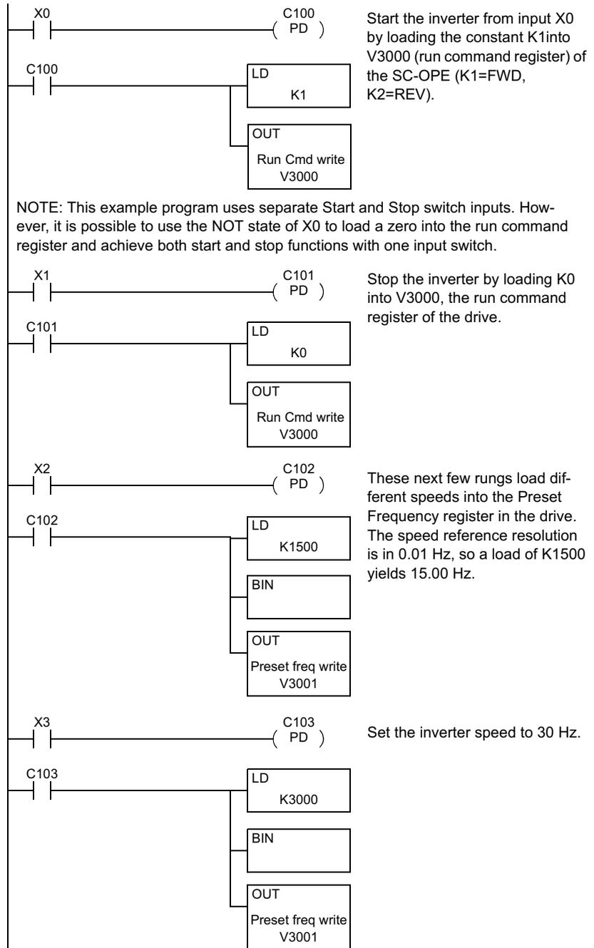
NOTE: This example program uses separate Start and Stop switch inputs. However, it is possible to use the NOT state of X0 to load a zero into the run command register and achieve both start and stop functions with one input switch.
