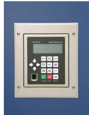
**9** Secure the SC-OPE to the bezel/housing with the two 3-38 x 1" screws (included in the Bezel Kit).
