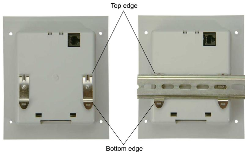
**7** Mount the SC-OPE to the DIN rail. First, hang the tops of the DIN rail clips over the top edge of the rail. Then push inward on the lower part of the bezel/housing to latch the SC-OPE to the DIN rail.
