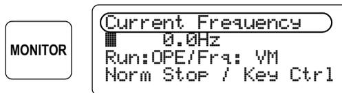
When the source of Frequency Setting is the Operator Keypad (OPE), the second line becomes dedicated to displaying the set frequency and actual frequency (pre-configured variable 2 output is suppressed). This feature is useful to help machine operators avoid severe frequency over-shoot / undershoot when the set acceleration and deceleration rates are relatively low.
