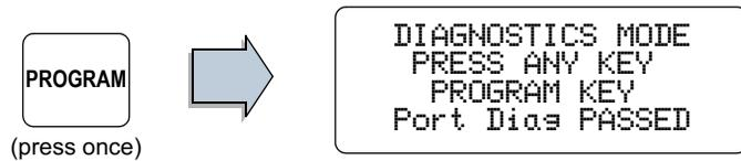
6 Returning to normal SC-OPE operation requires you to reset the SC-OPE. Press and hold the Mode key for 6 seconds; release it when the Startup Screen displays.
