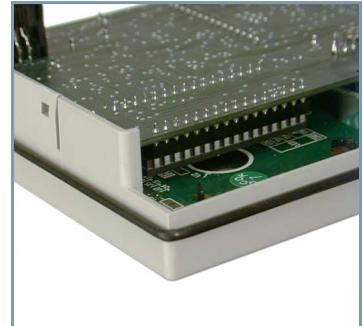
**8** Take the SC-OPE and tilt it into the bezel/housing opening in the panel, latching the bottom edge first as shown (below, left). Then push the top of the SC-OPE keypad to engage the upper latch (below, right).
