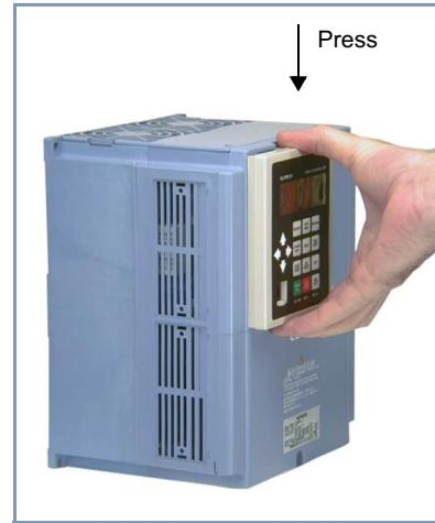
**8** Disengage the bottom retention latches and remove the SC-OPE uniformly in order to avoid mechanical binding.
