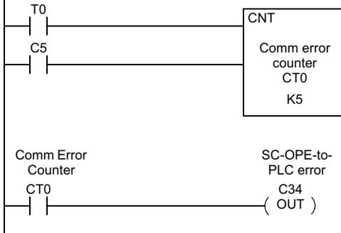
If errors persist, then increment the counter 5 times. When the counter is done, turn control relay C34 ON to record the error for SC-OPE-to-PLC communications. Control relay C5 turns ON once normal communication is resumed to reset the counter.
