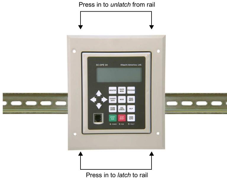
**8** Removal of the SC-OPE from the DIN rail is accomplished by pressing on the front top edge of the SC-OPE bezel/housing. This acts as a lever to unlatch the DIN rail clips at the bottom edge of the rail. This capability requires that the DIN rail be mounted securely to a solid surface as described in Step 1.
