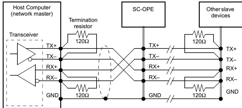
**Bias Resistors** A transceiver's differential signals are in a tri-state condition (floating, with respect to GND) between transmissions. This can make a network more susceptible to noise particularly with higher baud rates. The maximum speed of SC-OPE communications is 19.2 k Baud, still low enough for reliable communications in many applications. The Network Termination Board contains bias resistors. These include 1kΩ pull-up and pull-down resistors at each node.
