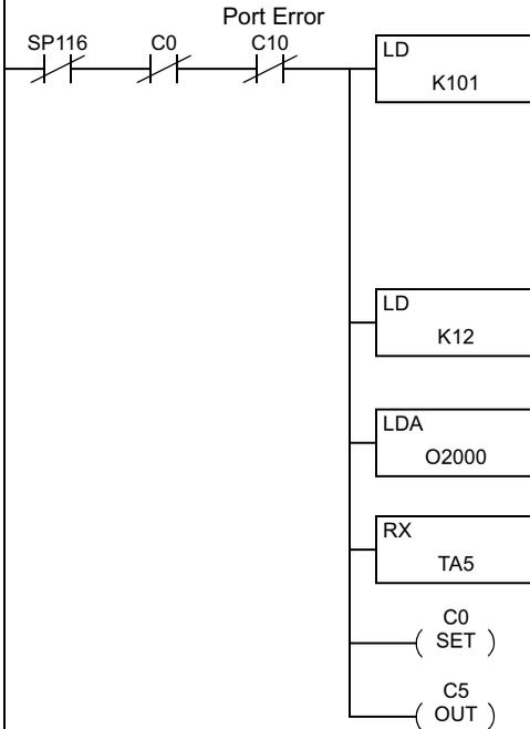
The LD box designates the bottom port of the DirectLogic CPU as master and specifies address 1 as the slave address. The last digit ("1") corresponds to the number of SC-OPEs (devices) on the network.
