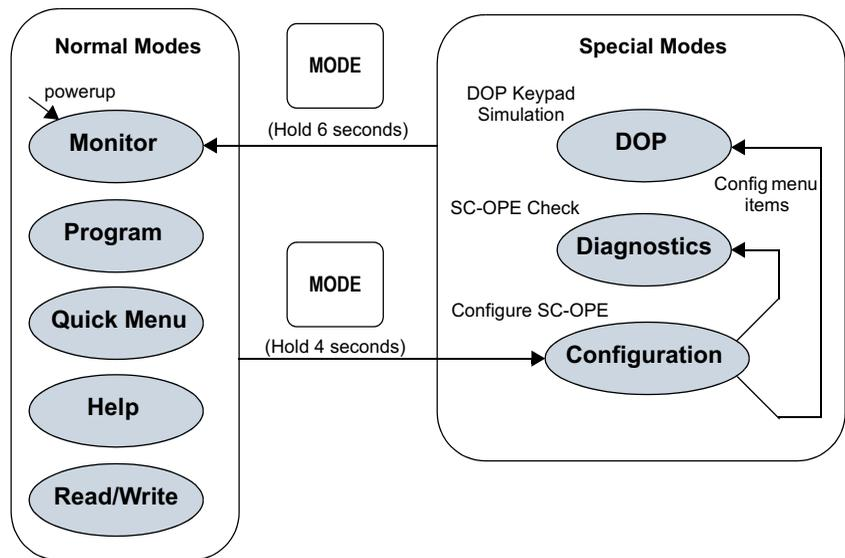
The diagram shows that the Mode key transitions the SC-OPE between Normal Modes and Special Modes, based on the duration of the Mode key press.
