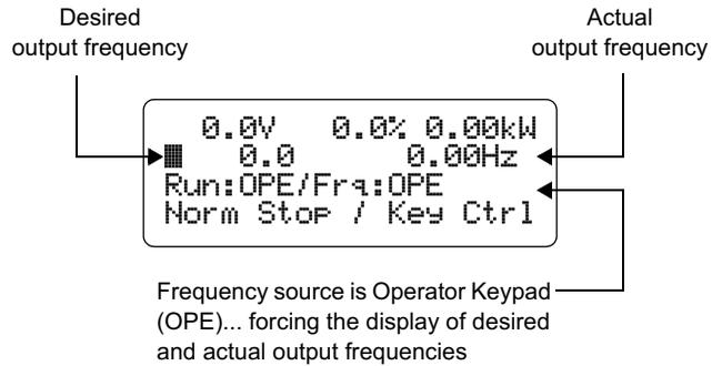
Program Mode provides access to change the four variables you can display on the upper two display lines. The figure below shows the location of the “Monitor Vars” submenu within the menu list in Program Mode.
