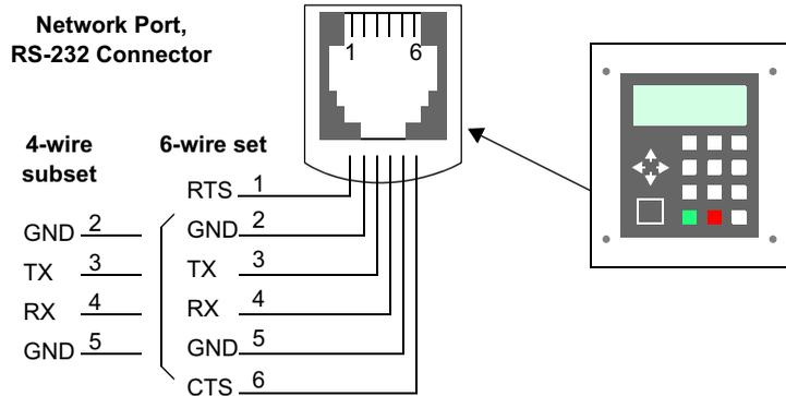
A typical RS-232 network port connection is between a PC and the SC-OPE only.
