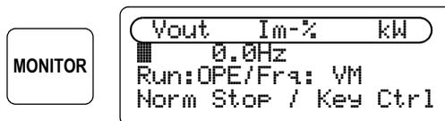
Press the Monitor Mode key again to view the name of the variable in position 2 (display line 2). Press the Monitor Mode key once more to return to the initial display.
