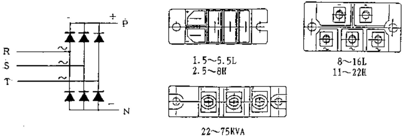
Converter module circuit diagram and top views
