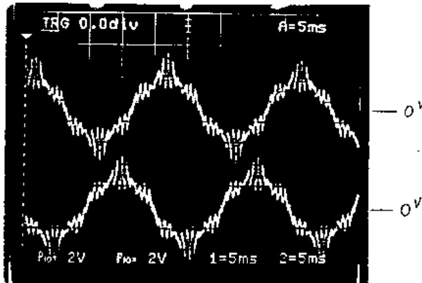
\* The waveform would be changed according to output frequency.
