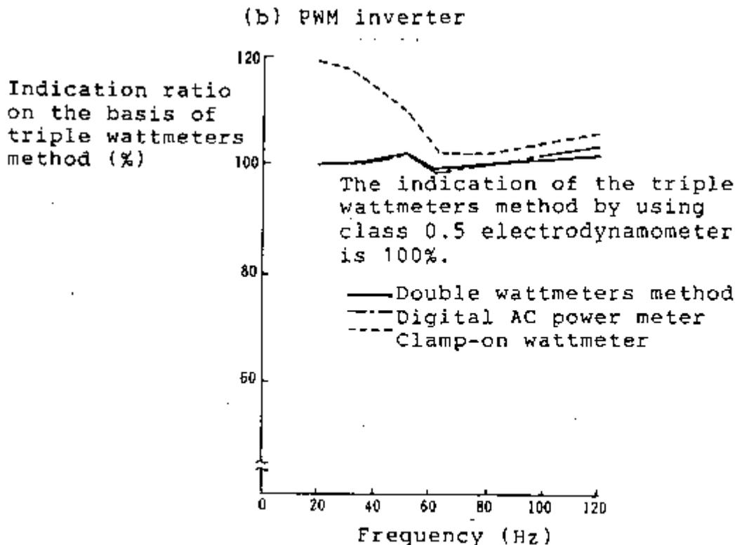
NOTE : Both (a) and (b) show the indication ratio as the indication of the triple wattmeters method is 100% while the torque is constant from 0Hz to 60Hz and the power is constant for more than 60Hz.
