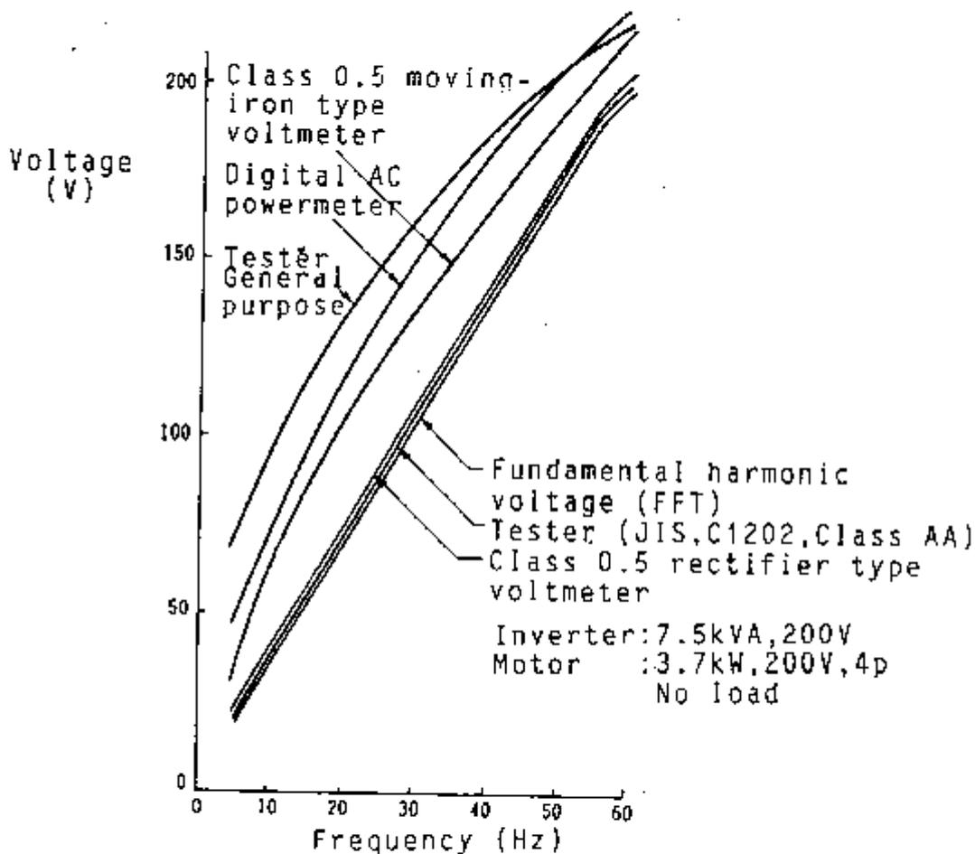
Fig. Measurement characteristics of output voltage of PAM inverter by using each instrument
