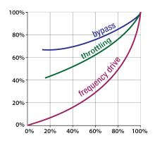
On the system curve shown above, a single performance curve shows the pump performing at a fixed speed. Fixed speed pumps draw nearly full horsepower consuming maximum energy full time, regardless of demand. When water is turned off
