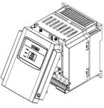
③ Move the wiring plate like shown below in case of wiring.
