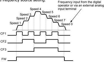
With multispeed binary operation mode, you can use the multistage speed determination time setting (C169) to specify a delay to be set until the relevant terminal input is determined. (time = C169\*10ms) Use this specification to prevent the application of fluctuating terminal input before it is determined.
