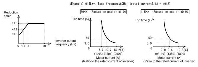
(c) Free setting of electronic thermal characteristic
