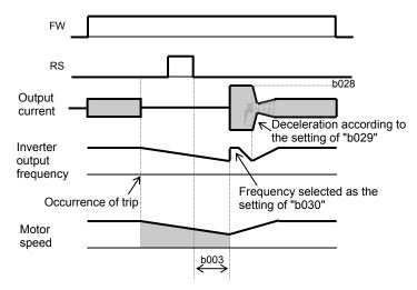
After the retry wait time (b003), the inverter restarts the motor with the frequency set as "b030". The inverter subsequently decelerates the motor according to the setting of "b029" while maintaining the output current at the level specified for "b029".
