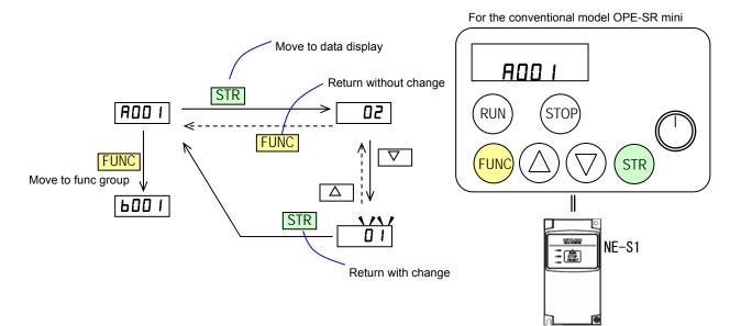
[Reference] Conventional inverter model and OPE-SR mini combination
