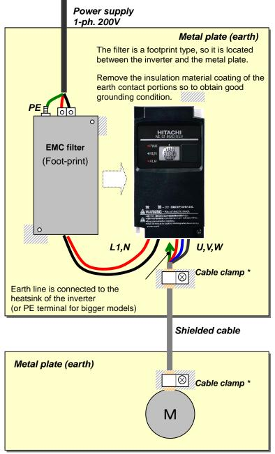
\*) Both earth portions of the shielded cable must be connected to the earth point by cable clamps. Input choke or equipment to reduce harmonic current is necessary for CE marking (IEC 61000-3-2 and IEC61000-3-4) from the harmonic current point of view, even conducted emission and radiated emission passed without the input choke.
