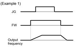
When "00", "01", or "02" is specified for the jog stop mode (A039), the jogging operation will not be performed if the FW signal is turned on earlier than the JG signal.
