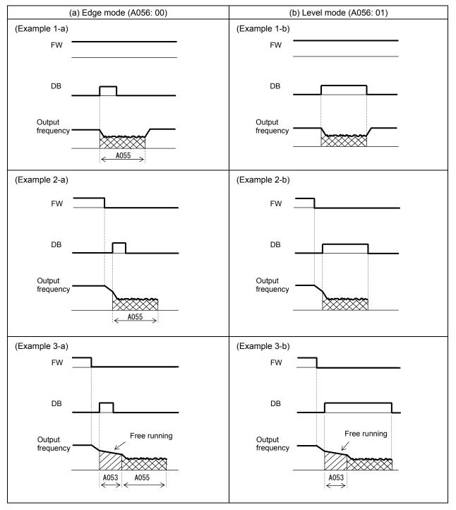
(3) Internal DC braking (A051: 01)
