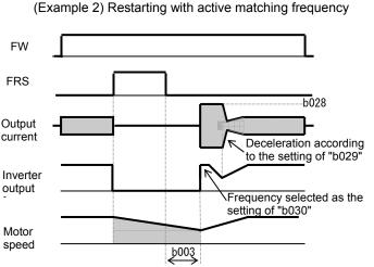
After the retry wait time (b003), the inverter restarts the motor with the frequency set as "b030". The inverter subsequently decelerates the motor according to the setting of "b029" while maintaining the output current at the level specified for "b029". When the output voltage matches the frequency, the inverter re-accelerates the motor up to the frequency that was set when the inverter shut off the output to the motor before the restart.
