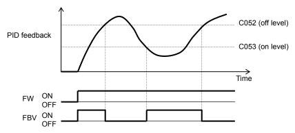
(11) Process variable (PV), PID feedback monitoring (d004)
