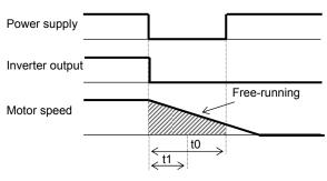
(Example 3) When the motor frequency (speed) is more than the setting of "b007" (b030=00):
