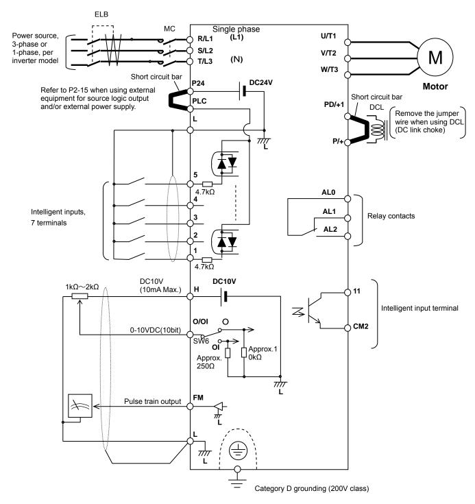
Note 1) Above shows an example of voltage (O) input. Changeover of SW6 must be done in case of current (OI) input.
