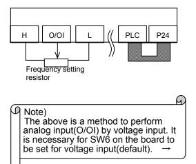
(3) <u>Method to perform driving in FW/RV teraminal and perform frequency setting in volume resistor</u> This is the operation method using Run command is given by intelligent input terminal such as FW(RV) function & Frequency setting is given by analog input such as O-L voltage. If you don't need to change such as Accel&Decel time, optional Operator is not required.) Below diagram is to set the external Freq. setting connecting H-O-L volume to supply O-L voltage.
