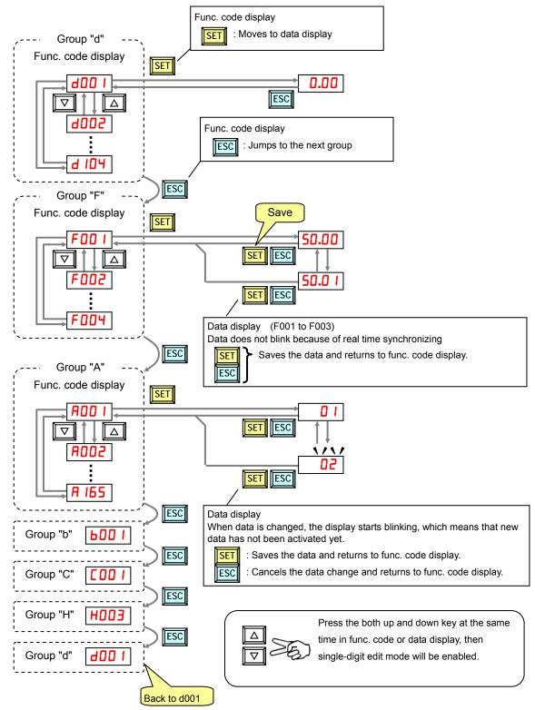
Note) Pressing the [ESC] key will make the display go to the top of next function group, regardless the display contents. (e.g.  $RO2 I \rightarrow [ESC] \rightarrow bOO I$ )
