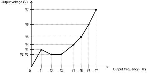
\*1 Even if 300 V is set as a free-setting V/f voltage (1 to 7), the inverter output voltage cannot exceed the inverter input voltage or that specified by the AVR voltage select. Carefully note that selecting an inappropriate control system (V/f characteristic) may result in overcurrent during motor acceleration or deceleration or vibration of the motor or other machine driven by the inverter.
