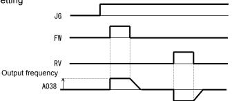
Since the inverter operates the motor with a full voltage for the jogging operation, the inverter can easily trip during the latter. Adjust the jog frequency setting (A038) properly so that the inverter will not trip.
