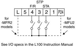
• If you do not assign the [F/R] intelligent input terminal, the three-wire operation will be limited to the forward direction only.
