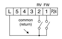
Each wiring example in this section shows both the -xMFU2 and -xMFR2 input wiring *in the same diagram*, as shown to the right. DO NOT connect terminal [P24] to [L]. Be sure the return terminal used matches your inverter type.
