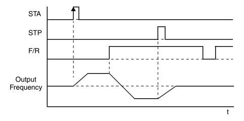
When both STA and STP signals are ON, the STP signal has priority (motor output will be OFF). However, the motor output resumes after STP signal is no longer active if the STA input is still ON.
