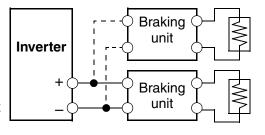
Use one BRD–E2 braking unit for the braking torque listed in the following table.
