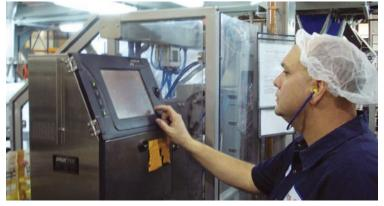
parts, a unique and innovative ink circulation system that helps reduce fluid evaporation, self-cleaning nozzles and gutters, and an IP55-rated stainless steel enclosure for protection against dust and moisture. These features also contributed to the BestSweet unit's stellar maintenance record.
