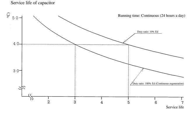
Appendix Figure 1 Ambient Temperature vs. Capacitor Life characteristics
