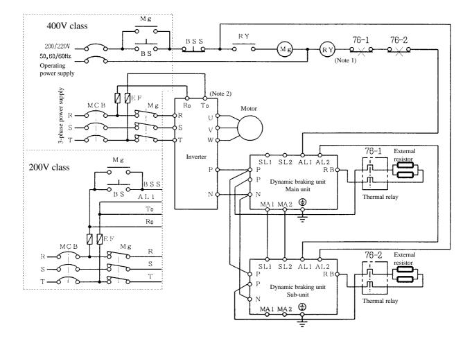
Note 1: Select relay RY according to the coil (Mg) specifications and the contact (RY) specifications. Note 2: R0, T0 terminals depend on inverter model.
