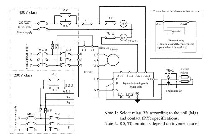
Figure 4.1 External connection example
