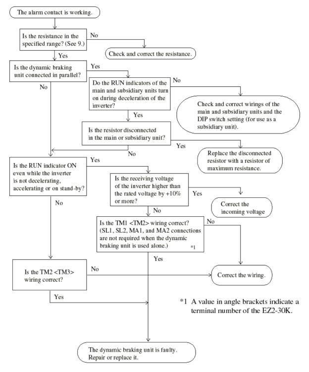
5.2 When the inverter is tripped by overvoltage during inverter deceleration This event may be caused by too much regeneration energy, which is unable to handle the increase in voltage.
