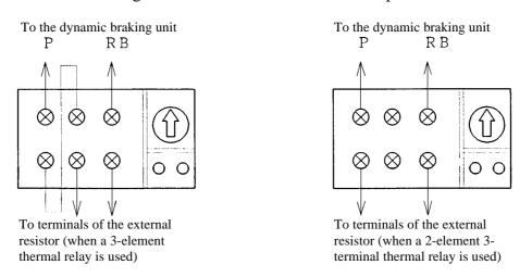
Figure 4.2 Connection of a Thermal Relay
