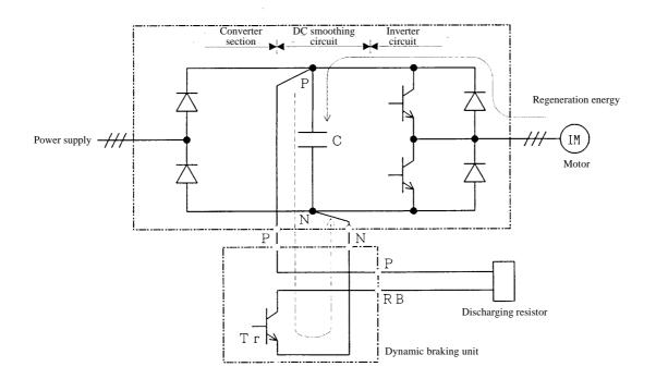
Figure 9.3 Dynamic braking by the inverter
