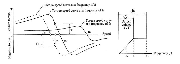
Fig. 8.1 Frequency Change and Motor Torque
