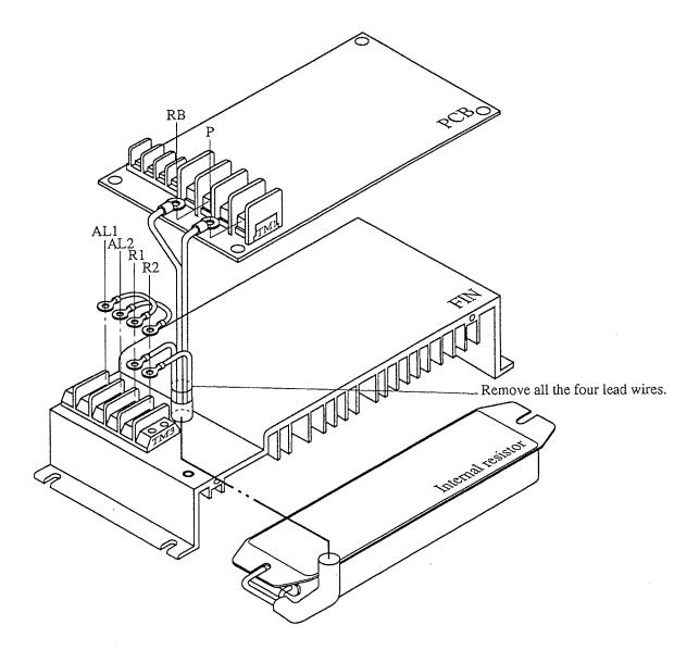
Fig. 2.1 How to Remove Internal Resistors
