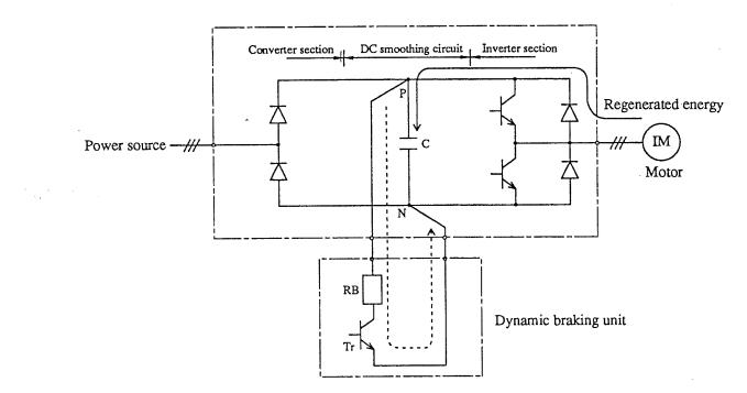
Fig. 8.3 Dynamic Braking by the Inverter
