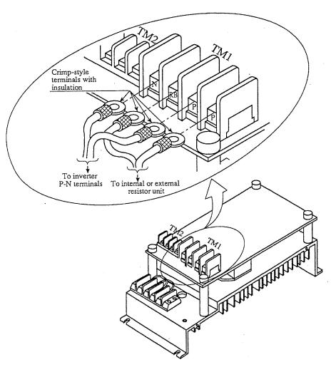
Fig. 4.1 Terminal Block Connection
