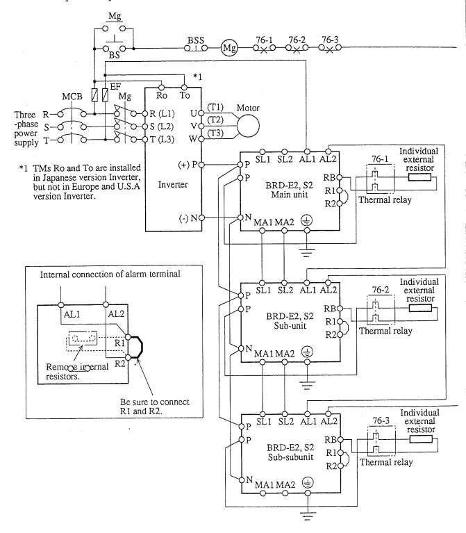
Fig. 4.6 Connection When Individual External Resistors are Used
